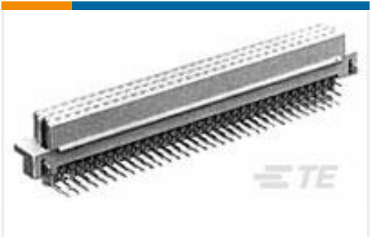
TE Part #5650875-5 ASSY,RECEPTACLE,EUROCARD,TYPE
